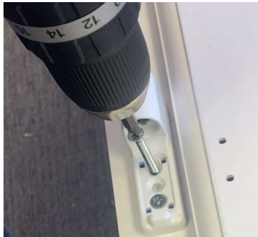
Secure hinge base to the door frame using 3 x (see recommended screws) Ø4.8mm screws.
