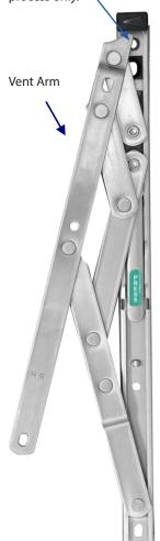
End cap must butt into the corner of the frame; this is particularly important for egress and high security products. The corner of the vent or weld sprue must not foul the end cap of the hinge.
